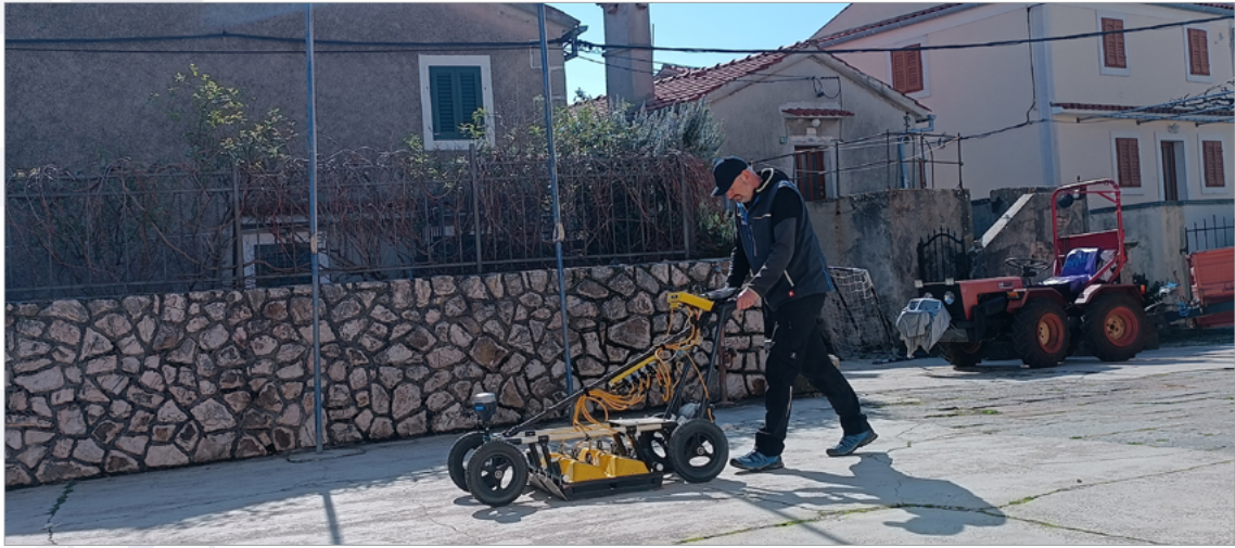
Figure 5: A Geophysical Survey of the Main Square in Beli with a Handheld Ground-Penetrating Radar System (elaborated by Nives Doneus, 2024)
