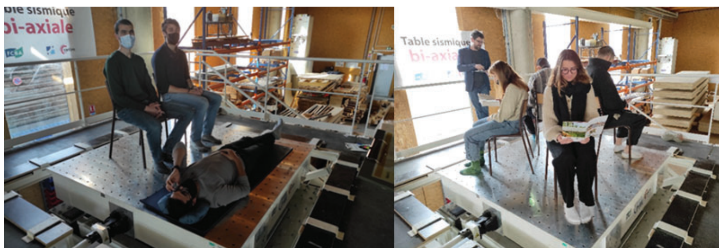
Figure 1: Experimental tests of vibrational comfort using a shaking table.
