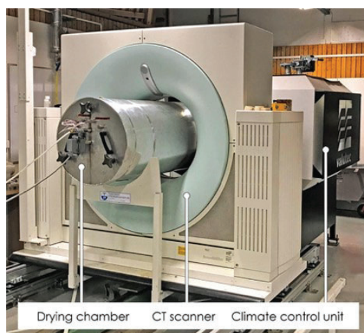
Figure 3: X-ray CT scanner and drying kiln fitted in the gantry of the scanner
